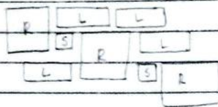
(Uncoursed square Rubble)
